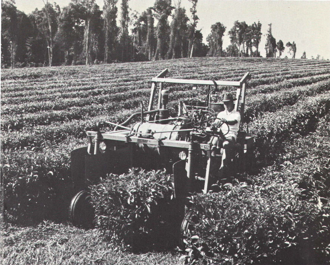
Spraying tea bushes for weed control by a machine that can be converted for harvesting
